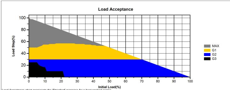
Load Acceptance chart represents the 'Standard' response for a heat soaked engine
